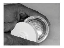
4. Replace lens insert with tool. Tighten to align tool with notch.
