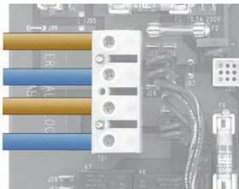
Remove the white wire connecting pins J26 and J23, then insert the second set of incoming wires provided.
