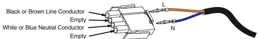
Note: A special tool is required to remove the pins from the connector body once they are snapped in place. Check with your Balboa Account Manager for information on purchasing a pin-removal tool.
