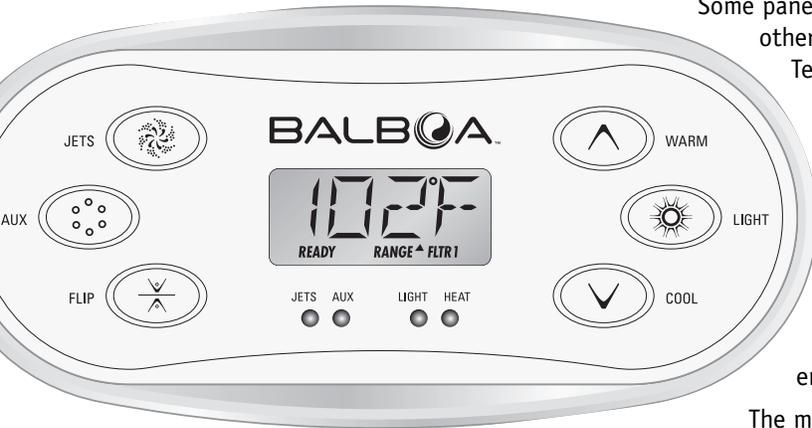
Some panels have separate **WARM** (Up) and **COOL** (Down) buttons, while others have a single **Temperature** button. In the navigation diagrams Temperature buttons are indicated by a single button icon.
