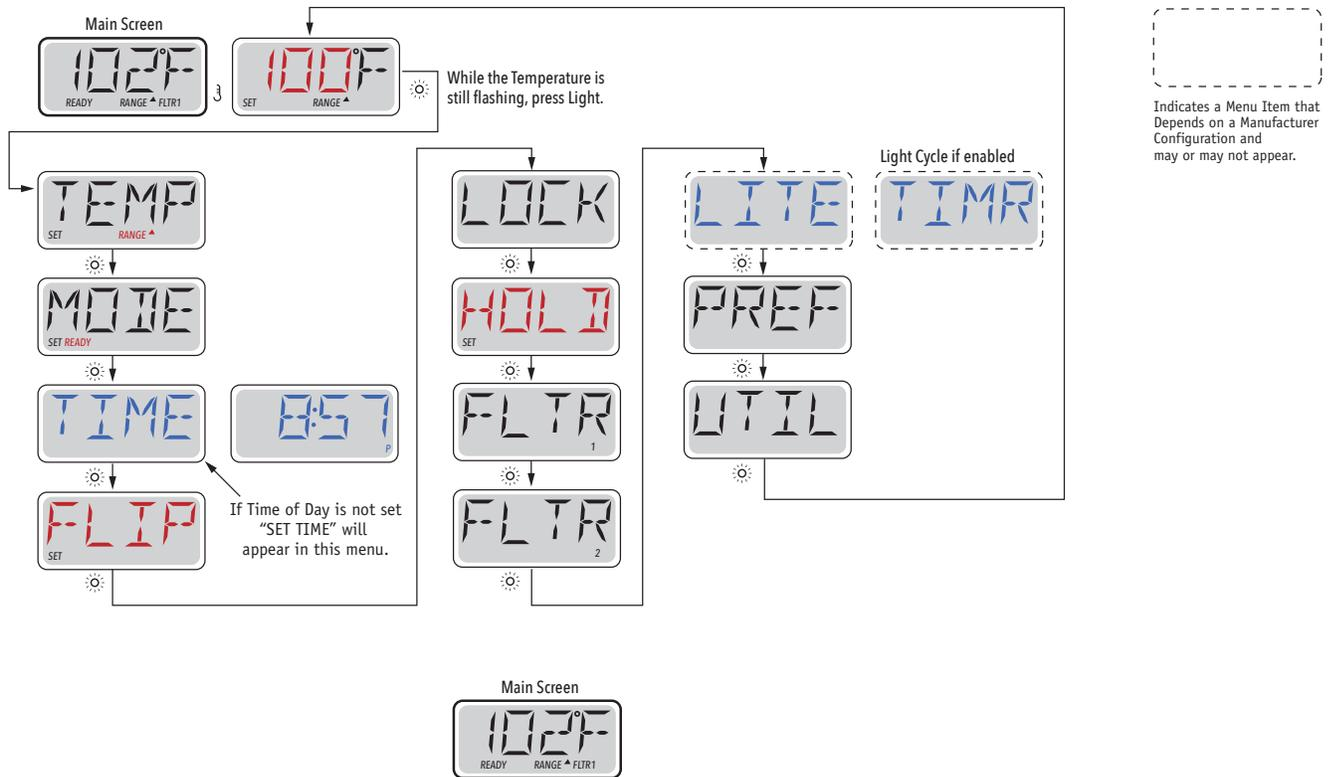
Waiting a few seconds in the Main Menu will allow the display to revert to the Main Screen. Most changes are not saved unless Light ☀ is pressed. Refer to key above.
