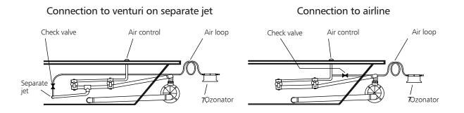
It is recommendable to activate the ozonator together with a therapy pump in a whirlpool or together with a filtration pump on a spa.
