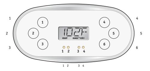
In all Setups, the button labeled "AUX" on overlay 13579 (shown below) controls Jets 4. In Setups 2, 4, 7 (which have a Blower), an AX10A3 auxiliary panel plugged into J5 (Bank 1) must be used to control the Blower.
