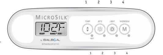
The TP400T is mainly suitable for Setup 12. In Setup 11 an AX10 A3 for Blower will be required. The TP400T is not supported in Setups 1 - 10 which have a Pump 2.
